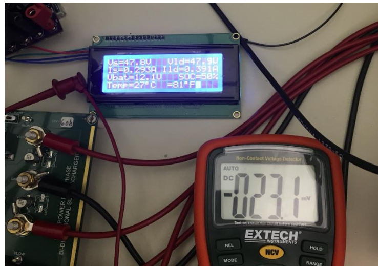
Figure 5-8: LCD Output and BUCK Signal for BOOST Mode of Operation
