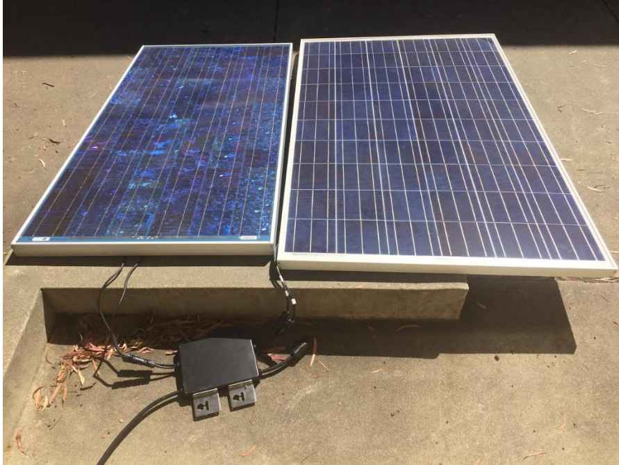
Figure 5 - 5: Microinverter and solar panel setup for 240V outlet
