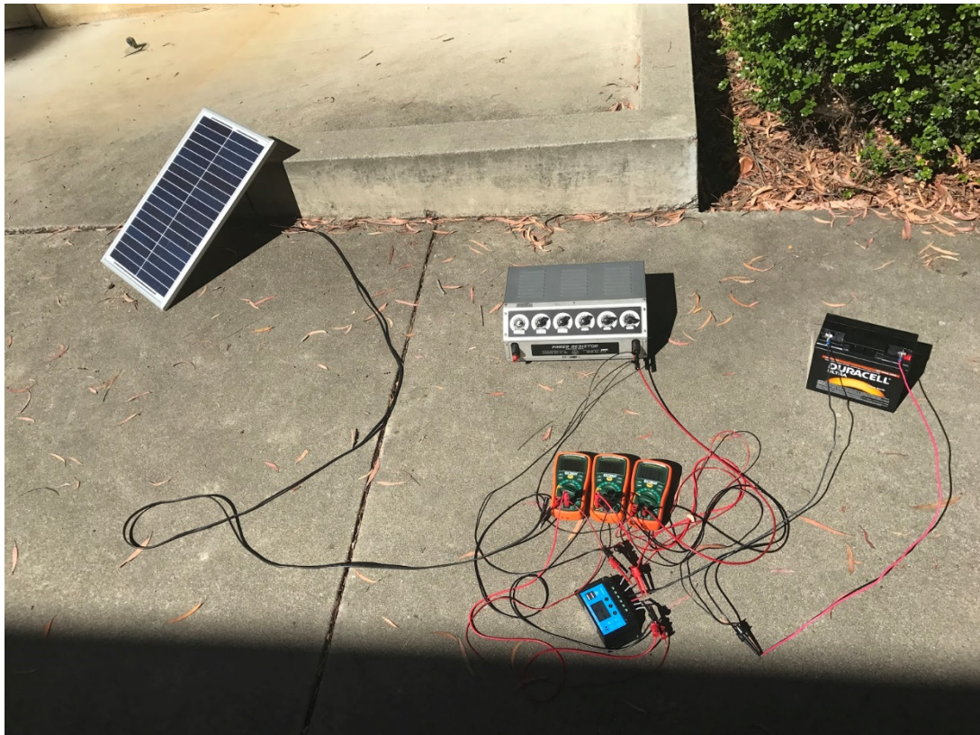
Figure 5-8. Test Setup for Charge Controller and Battery
