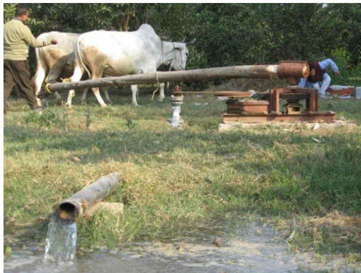
Figure 1-3. Example animal driven water pump with gear box and bullocks [4]
