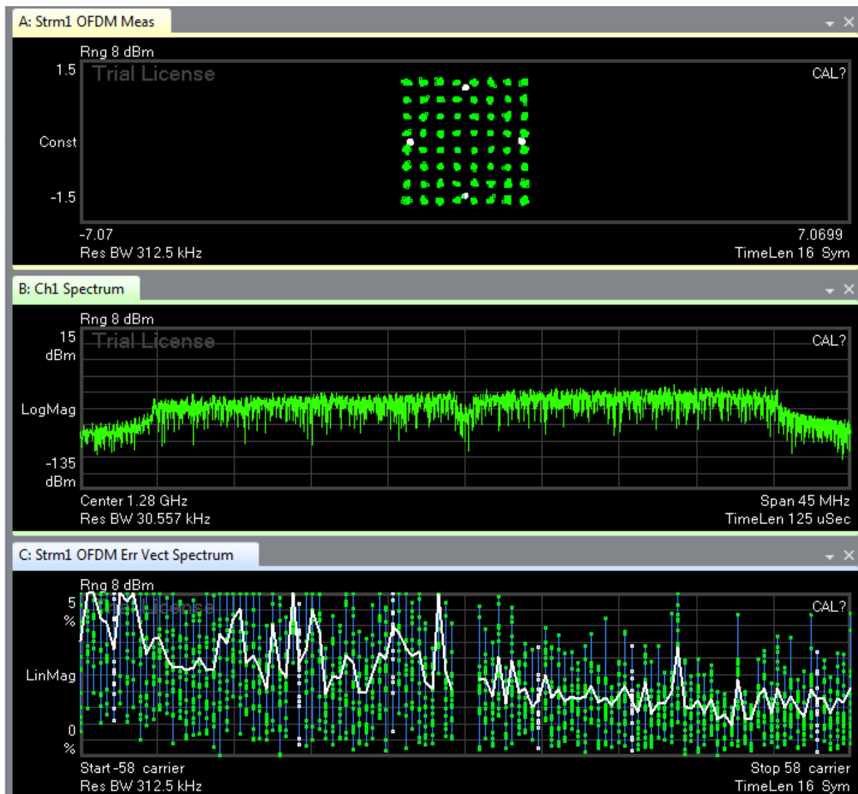
Figure 4.3: An instance of the IQ diagram, spectrum analyzer view, error vector spectrum are displayed.
