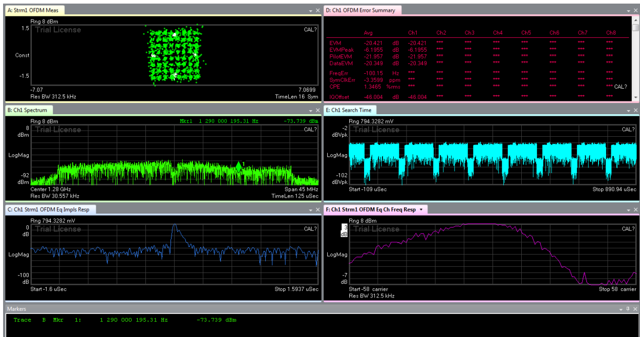
Figure 4.33: MISO 16 cm separation case where antennas are back-to-back, front antenna is 1 m away receivers centroid. EVM is -20.421 dB.
