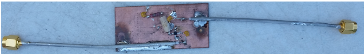
Figure 3.40: ERA-3+ first prototype implementation.
