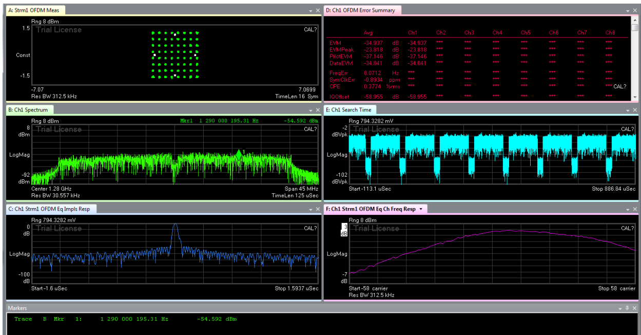
Figure 4.30: MISO 10 cm horizontal separation case. EVM is -30.932 dB.
