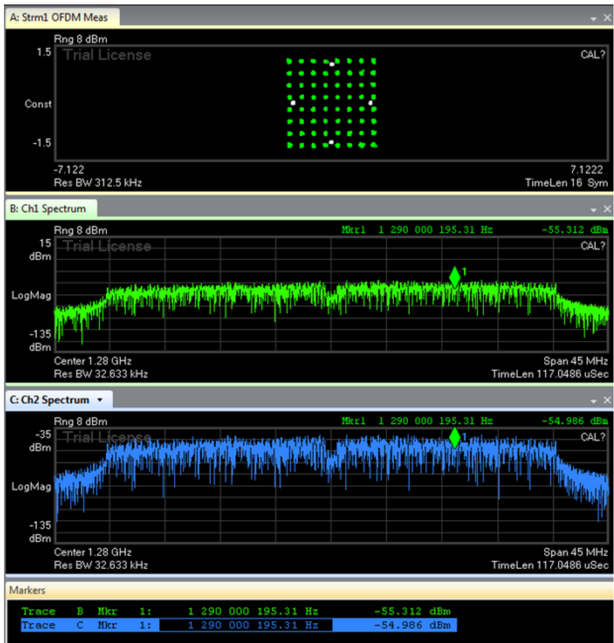
Figure 4.36: SIMO test case results. IQ diagram, spectrum analyzer view, error vector spectrum are displayed.
