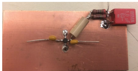
Figure 3.42: ERA-3+ second prototype implementation underway; only the semi-rigid coax cables need to be soldered on.
