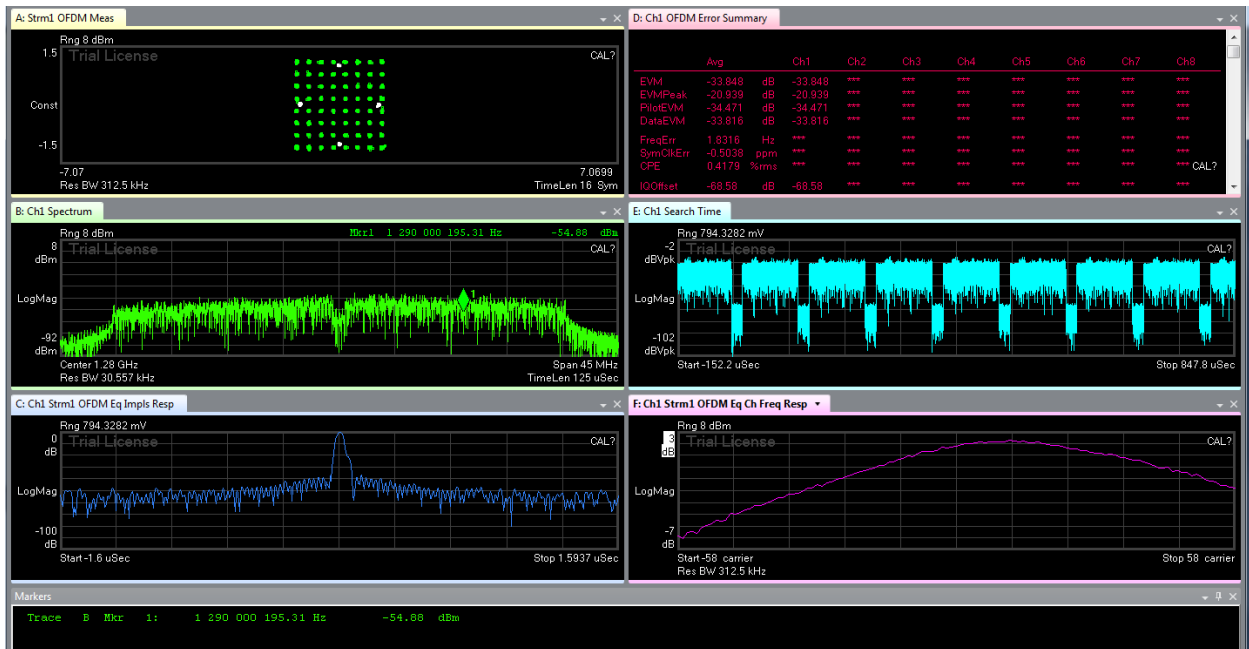
Figure 4.31: MISO 40 cm horizontal separation case. EVM is -33.848 dB.
