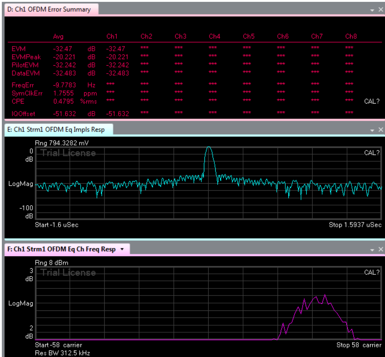
Figure 4.6: The second instance of error vector summary, impulse response, and channel frequency response are displayed. The error vector magnitude reads -32.47 dB.
