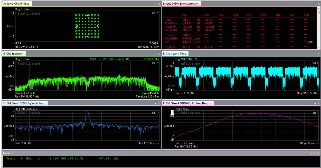
Figure 4.32: MISO no separation case where antennas are back-to-back, front antenna is 1 m away from receivers' centroid. EVM is -31.551 dB.
