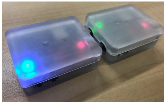
FIGURE XXV PACKAGED TRANSMITTING AND RECEIVING UNIT
