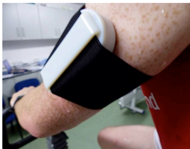
Figure 4-5: SWEATCH device in place on a volunteer's arm during a trial on a stationary exercise bicycle.
