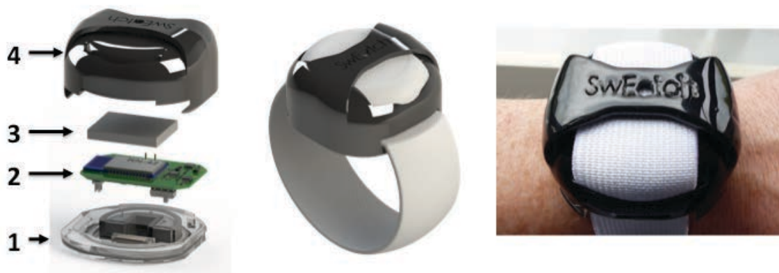
Figure 5-1: Improved SWEATCH ‘watch’ type platform with a render (left) showing the individual components including; fluidics and potentiometric sensing (1), electronics (2), lithium polymer battery (3) and 3D-printed housing beside a render of the enclosed system (left) with strap and a photo of the realised device (right)
