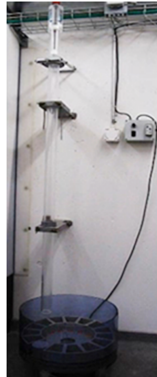
Figure 2. Settling tube apparatus used in this study. Detailed technical and operation information has been reported in Hu et al. (2013).
