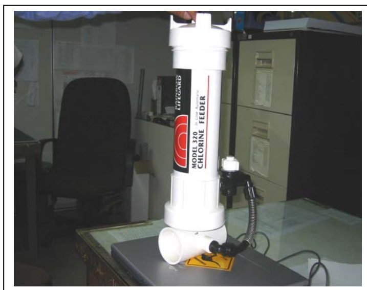
Figure 30 – The Klorman Chlorine Dispenser Unit
