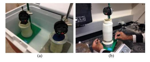
Figure 4.3 (a) Inundation of Soil Sample in Water Bath; (b) Measurement of Radial Swell using "Pi Tape."
