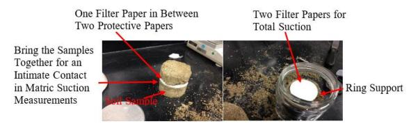
Figure 4.1 (a) Matric Suction (left) and Total Suction (right) Measurements
