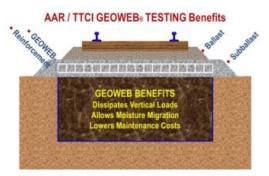
Figure 1.2 Schematic of Railroad Track Structure Comprising a Geocell-Reinforced Subballast Layer (AAR/TTCI, 2012).
