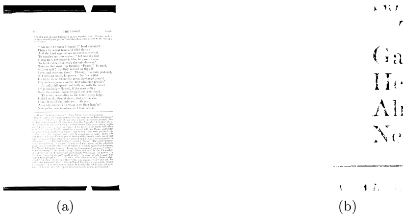
Figure 2.5: a) Global threshold of > 80 was performed, b) Enlarged view of mark area
