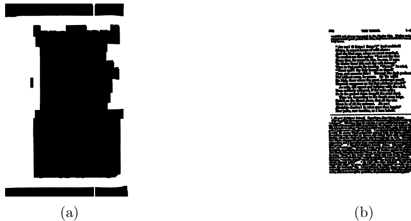
Figure 2.6: a) Dilation: 255 \times 255 structuring element, b) Dilation with 25 \times 25 structuring element
