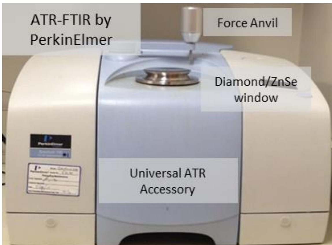
Figure 2.2. Perkin Elmer spectrum 100 FTIR Spectrometer equipped with U-ATR accessory (with components labeled). This instrument was used for the analysis of the cyanide supernatant and polymer produced from several heated ammonium cyanide reactions.
