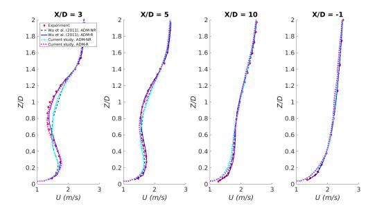
Figure 5.9: Streamwise velocity profiles wind turbine wind tunnel experiment and simulations. Z/D refers to height above ground level normalized by the turbine diameter. Results are shown from the wind tunnel experiment from Chamorro and Porté-Agel [12], ADM-NR and ADM-R simulations [71], and the ADM-NR and ADM-R results from the current study using GIN3D. The velocity profiles are at 3D (3 diameters), 5D, and 10D downstream as well as 1D upstream.
