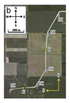
Figure 5.10: Wind turbine and SODAR station locations for the subset of the wind farm in Mower County. S1 and S2 represent SODAR stations and T39-T43 represent turbines. Image is adopted from [50].
