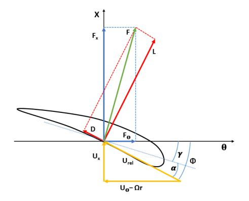
Figure 4.4: Visualization of an airfoil cross-section showing the relative forces, angles, and velocities for the BEM approach.  $\gamma$  is the local pitch angle,  $\alpha$  is the angle of attack, and  $\phi$  is the angle of relative wind at which  $U_{rel}$  approaches. Image is adapted from [50].
