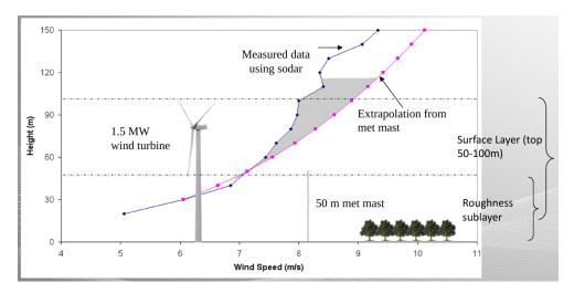
Figure 2.2: Observed difference between mast extrapolation and SODAR measurements. Image is adopted from AWS TruePower, a UL Company. [8]
