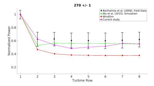
Figure 5.21: Average power at each turbine row normalized by power at row 1. Field data is reported in Barthelmie et al. [4] and the previous ADM-R simulation and WindSim [70] industry software results are reported in Wu et al. [72].
