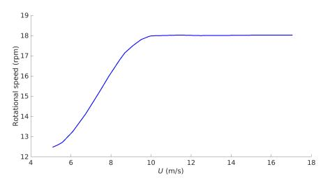
Figure 5.20: Reported angular speed as a function of wind speed for the Vestas V80 turbine. Data is from [72].
