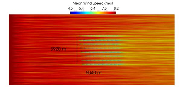
Figure 5.16: Visualization of the Horns Rev wind farm mean flow field showing the wind farm dimensions.
