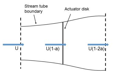
Figure 4.2: Visualization of the stream tube boundary around the actuator disk showing the fractional relationship between incoming velocity and the axial induction factor. Image is adapted from [34].
