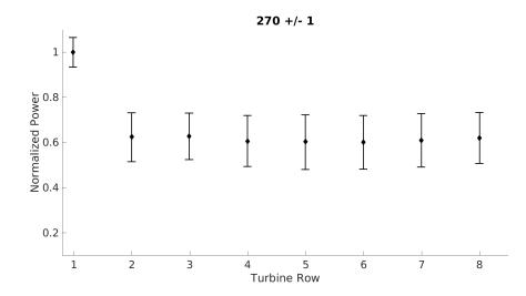
Figure 1.4: Normalized turbine power for each row of Horns Rev wind farm when the flow direction is aligned with turbine rows. Data is from [5]. The X-axis displays the turbine row and the Y-axis measures power normalized by power at the first row.
