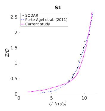
Figure 5.13: Streamwise velocity profiles at SODAR station S1 in the Mower County. Results are shown for the SODAR stations, Porté-Agel et al. simulation [50], the log-law profile, and the current study simulations performed with GIN3D using the turbulent perturbation inflow method.
