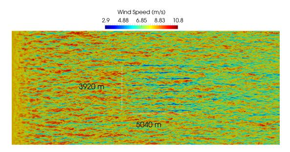
Figure 5.17: Visualization of the Horns Rev wind farm instantaneous flow field showing the wind farm dimensions.
