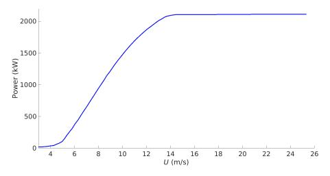
Figure 4.1: Plot of power as a function of wind speed for the Suzlon S88-2.1 MW wind turbine. Data is from [62].
