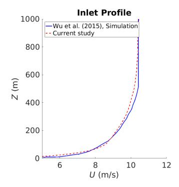
Figure 5.15: Incoming velocity profile for the Horns Rev wind farm showing the current study and the velocity profile in Wu et al. [72].
