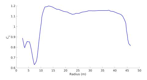
Figure 5.11:  $C_L$  curve as a function of radius as reported from the 3D simulations in Laursen et al. [31]. Data is from [31].
