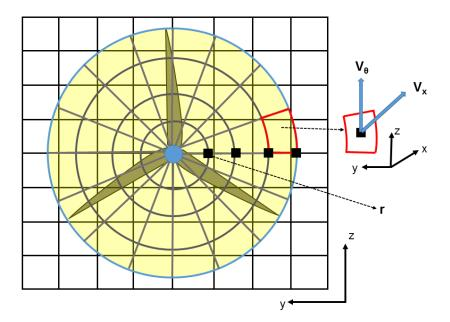
Figure 4.5: Visualization the blade element mesh overlaid on the Cartesian mesh.  $V_x$  and  $V_{\theta}$  are the axial and rotational components of the velocity, the uses of which are detailed in [34]. r is the radius at each blade element. Image is adapted from [72].
