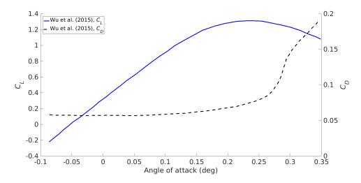
Figure 5.14:  $C_L$  and  $C_D$  curves as a function angle of attack as reported in [72]. Data is from [72].
