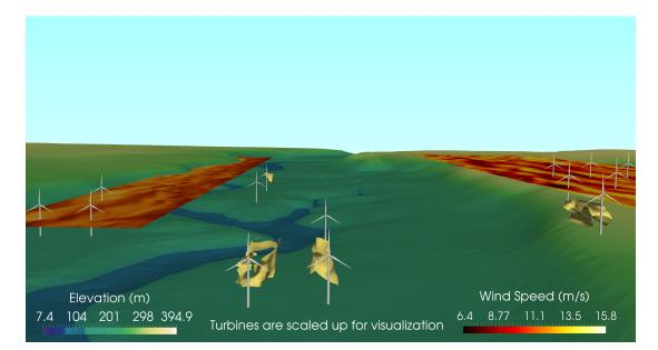
Figure 5.22: Visulization of the turbines, complex terrain, and flow field for a hypothetical wind farm in Hagerman, Idaho.
