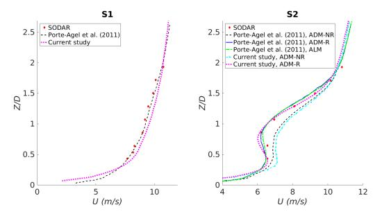
Figure 5.12: Streamwise velocity profile results showing simulation and field data results for the wind farm in Mower County. Results are shown for the SODAR stations, the ADM-NR, ADM-R, and ALM simulations from Porté-Agel [50], and the ADM-NR and ADM-R simulations performed with GIN3D.
