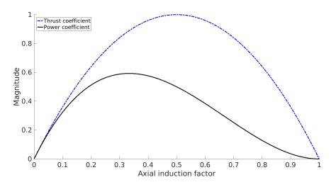
Figure 4.3: Plot showing the relationship between a and the thrust and power coefficients. Image is adapted from [34].
