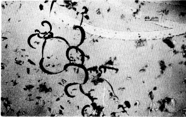
FIG. 9. Optical micrograph of silver deposit in glass E1 ion exchanged for 8 h \times 210 .
