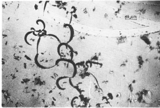
FIG. 9. Optical micrograph of silver deposit in glass E1 ion exchanged for 8 h \times 210.
