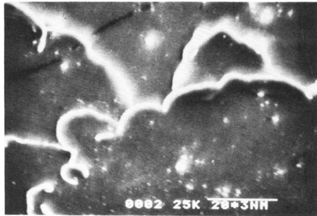
FIG. 11. Electron micrograph of silver deposit in glass F2 ion exchanged for 8 h \times 1500 .
