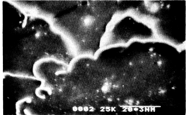
FIG. 11. Electron micrograph of silver deposit in glass F2 ion exchanged for 8 h \times 1500 .
