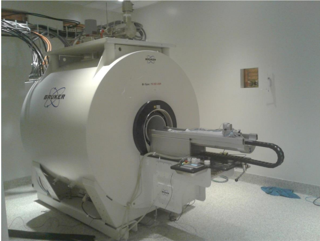
Figure 2-6: A 7 T Bruker small animal MRI scanner
