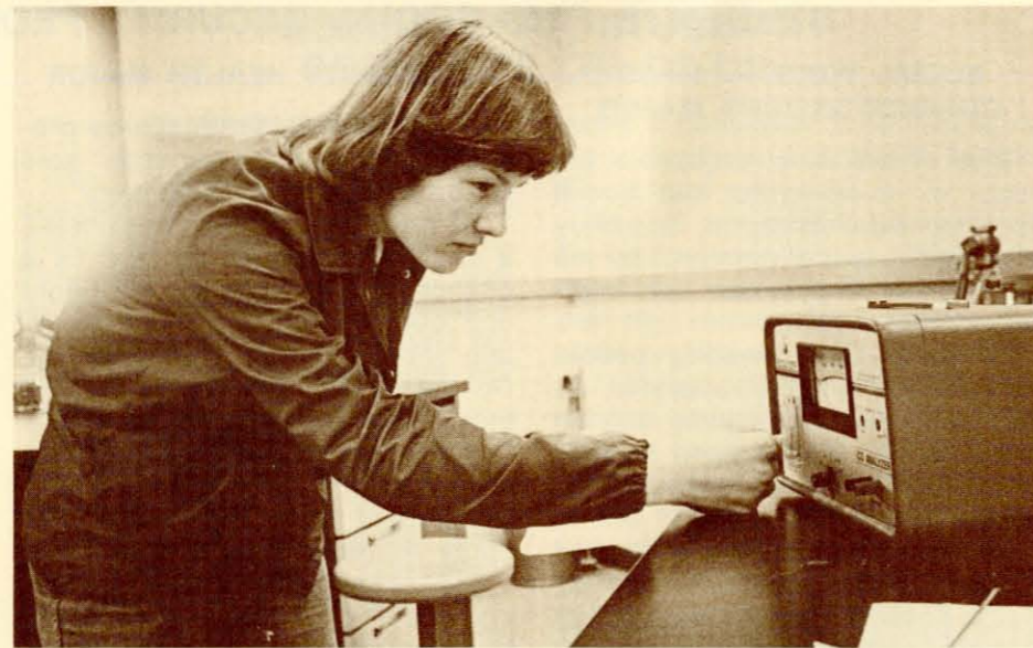
Cheryl (Runyon) Lucas operates an Ecolyzer, an instrument for measuring carbon monoxide.
