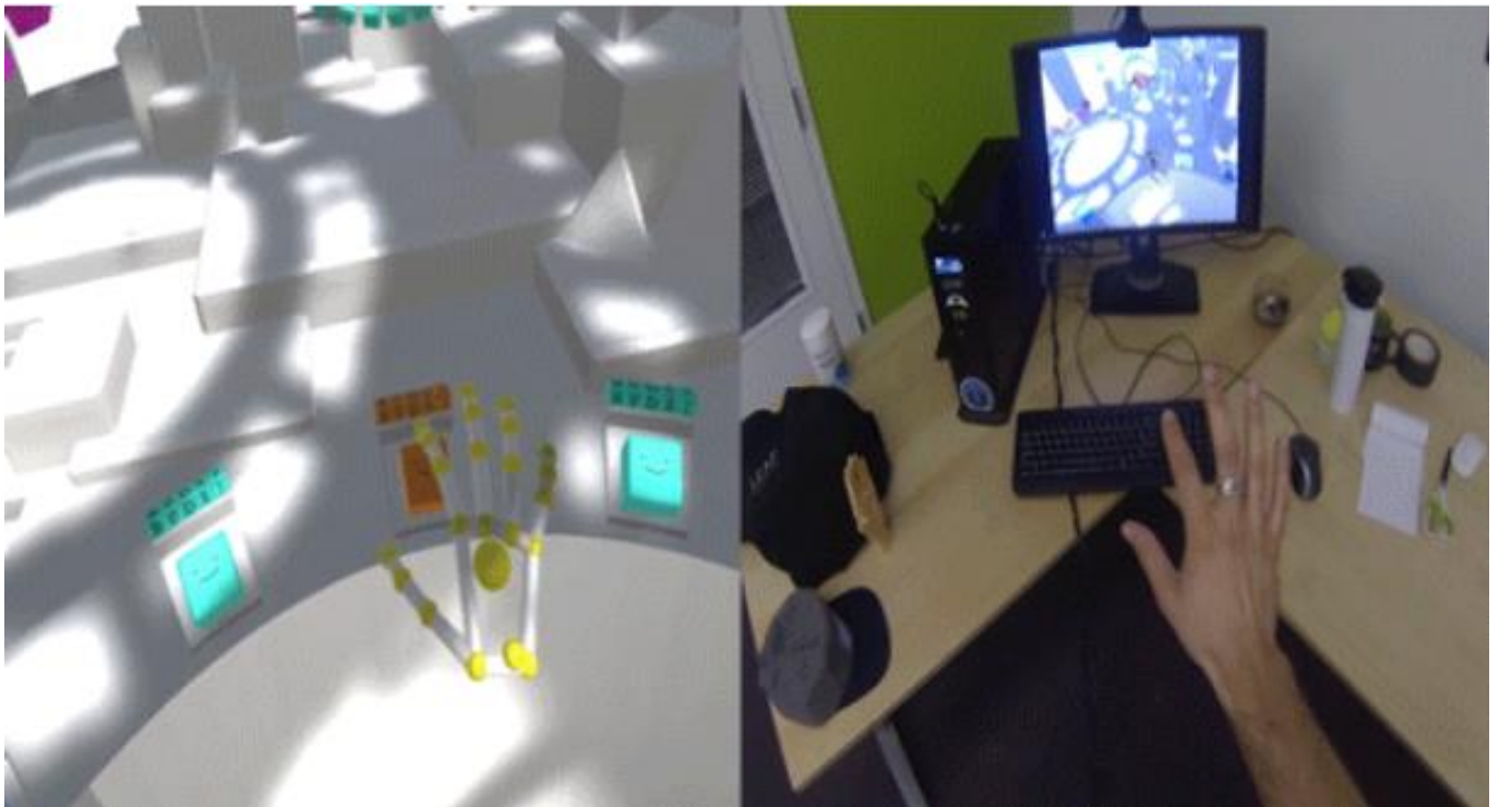
Figure 4 Bare hand input from Leapmotion
