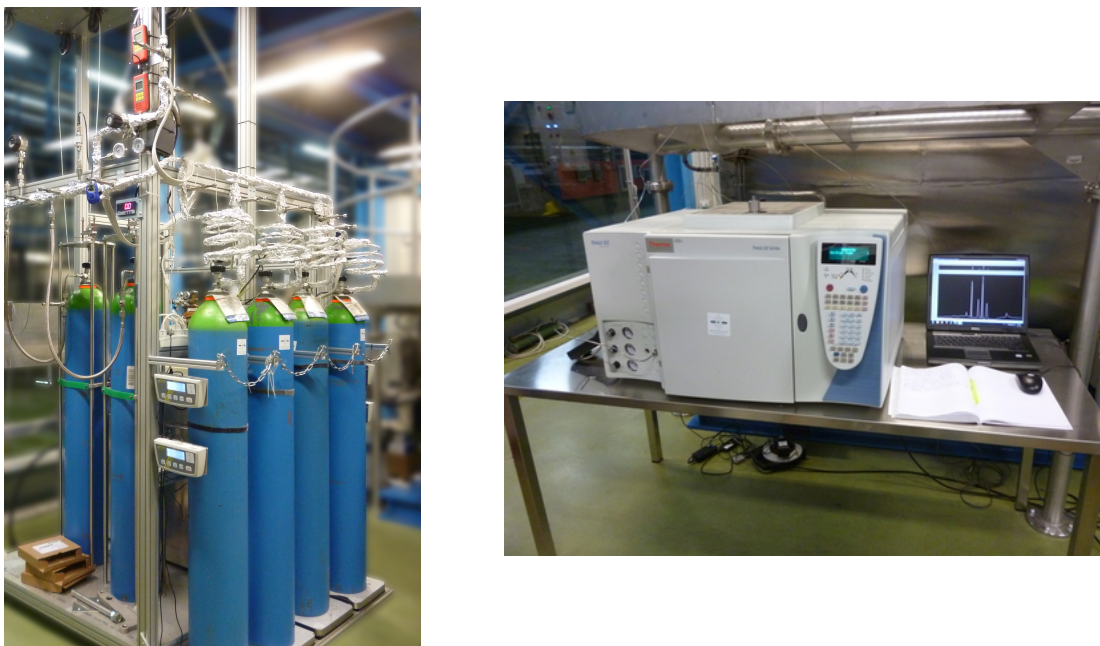
Figure 3.1: Pictures of the XENON1T bottle rack (left) and GC (right) as they are operated in the Gran Sasso Underground Laboratory.
