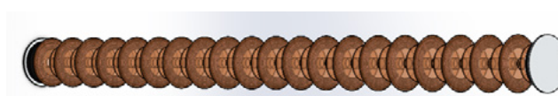
Fig. 7. Novel insulation string" with (i) High-Voltage insulation & (ii) Wireless Power Transfer capabilities [43], [44].
