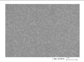
Figure 1: The SEM image showing the scaffold after the assembly of RADA16-I peptides.
