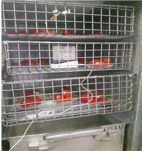
Fig. 3. Loaded Tomato postharvest storage system showing the experimental set up.
