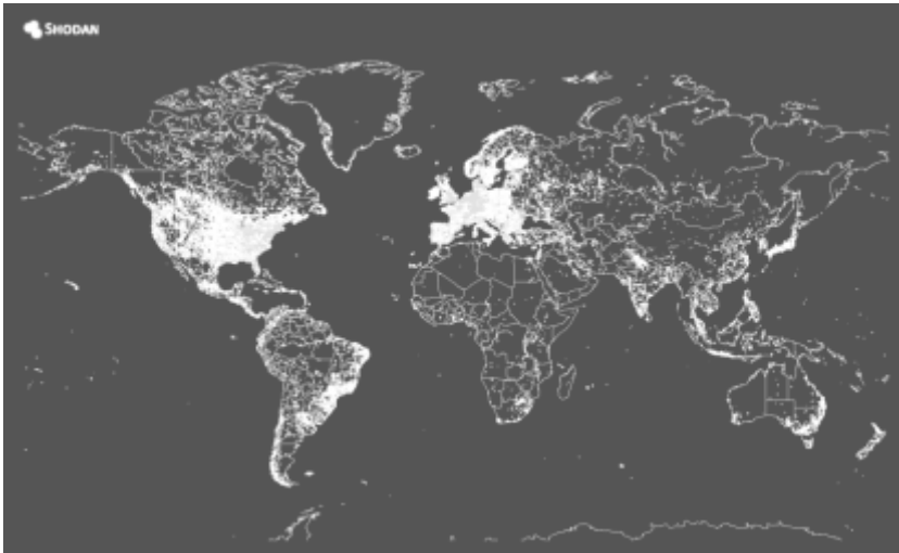
Figure 9: World map of 24-hour relative average utilization of IPv4 addresses observed using ICMP ping requests as part of the Internet Census of 2012 (Carna Botnet), June - October 2012. Key: from red (high), to yellow, green (average), light blue, and dark blue (low).
