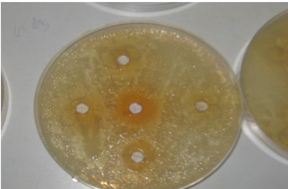
Plate 4.1: Inhibition zone of Ag nanoparticles formed using C. indica (AAg 0.5, 1.0, 2.0 and 3.0) against Staphylococcus aureus
