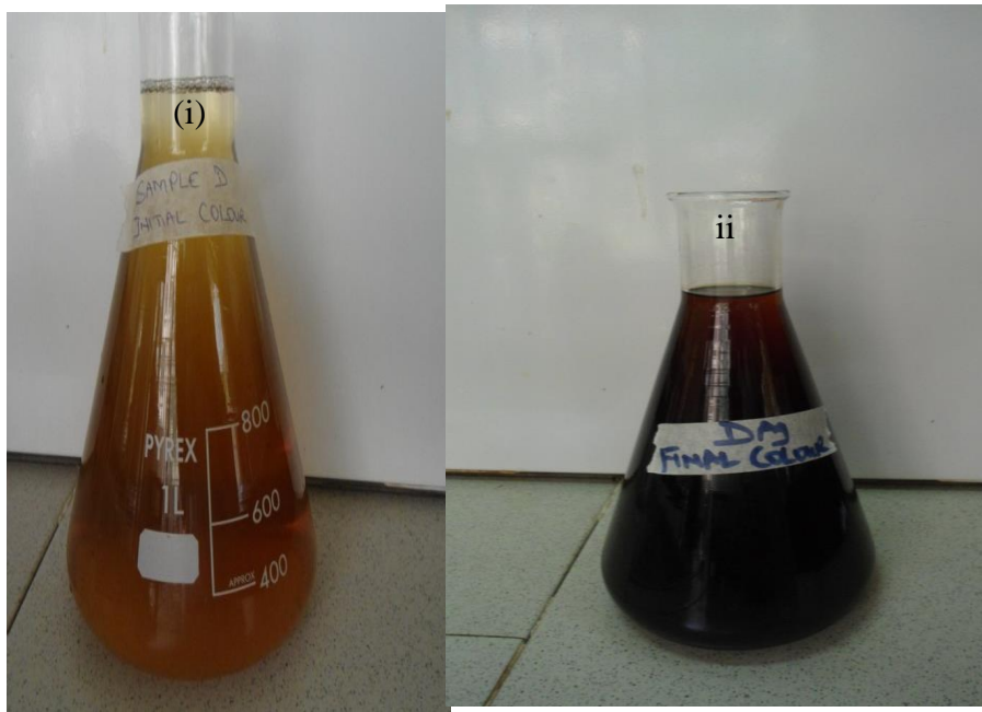
Figure 4.51e (i) = \text{AgNO}_3 solution with extract before reduction (ii) = Final silver dispersion formed after reduction
