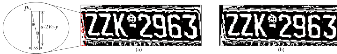
Figure 7 (a) NP image before vertical correction. (b) NP image after vertical correction.
