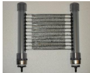
Figure 4: Metal foam heat exchanger of flat tube configuration
