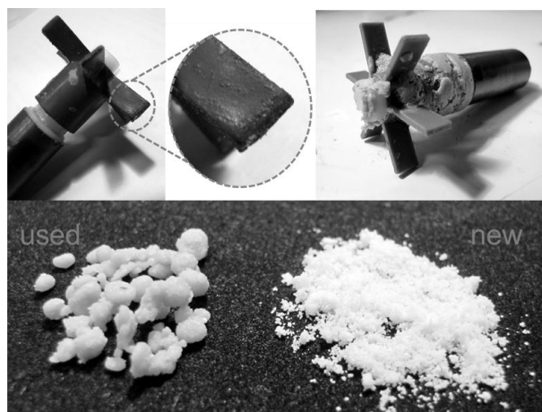
Figure 6: Abrasiveness and agglomeration of micro-encapsulated polystyrene-coated paraffin
