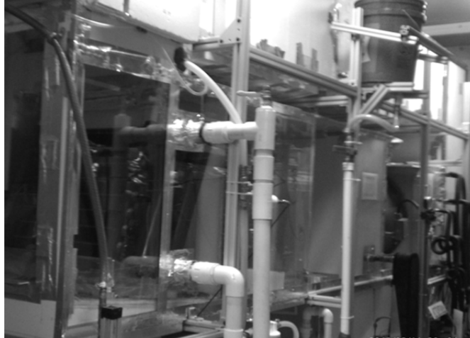
Figure 1: Experimental facility used for testing the condenser performance of round-tube louvered-fin heat exchanger in dry and wet conditions.
