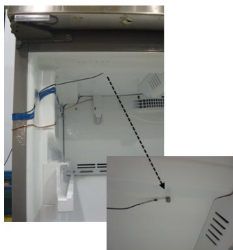
Figure 7: Accelerometer positioned at the top of the freezer liner
