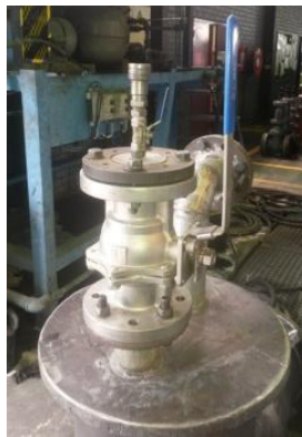
Fig. 2. 80NB intake ball valve
