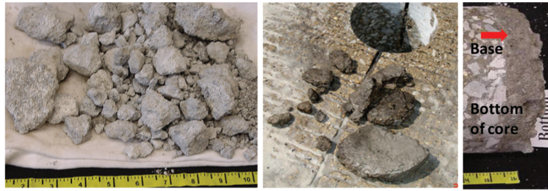
Figure 4.3 Examples of some of the base material cemented into larger chunks (left and center), and cemented onto the bottom of the core (right).
