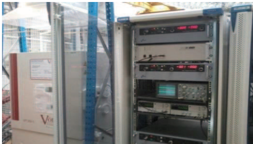
Fig. 2. Climatic chamber and power electronics as a test bench for the two types of insulation materials
