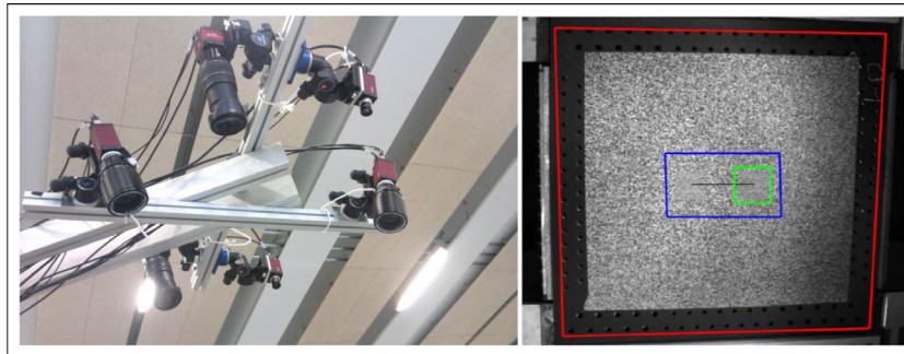
Fig. 5. Set of 6 cameras and areas covered on the specimen.
