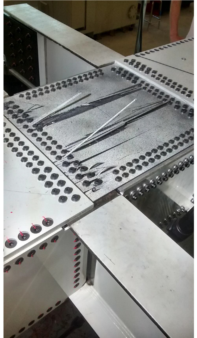
Fig. 17. Failure pattern of a thick notched composite specimen under tension.
