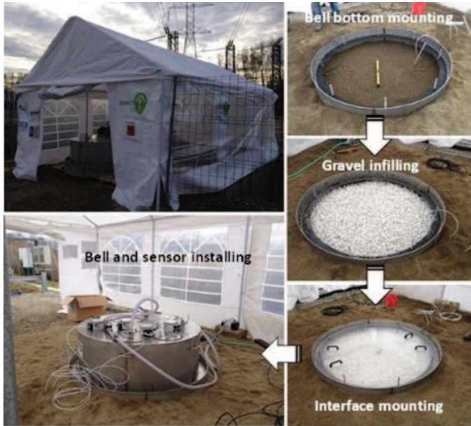
Figure 1 - View of the experimental set-up in the PISCO 2 facilities at Ponferrada. The sequence of pictures on right represents the installation of components.
