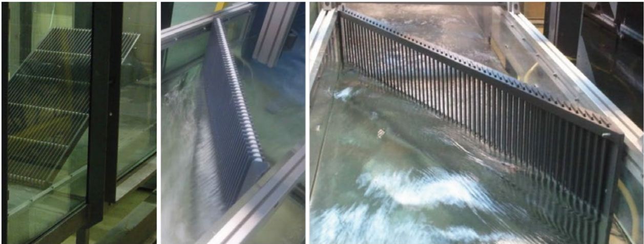
Figure 1: Different trashrack configurations tested. From left to right: inclined rack (observed from upstream), angled rack with perpendicular bars (observed from downstream) and angled rack with streamwise bars (observed from upstream).
