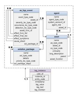
Figure 5: Failure Context in Asset Lifecycle Management (left) Failure Context (right) Metadata Extension ((Pistofidis et al. 2014))
