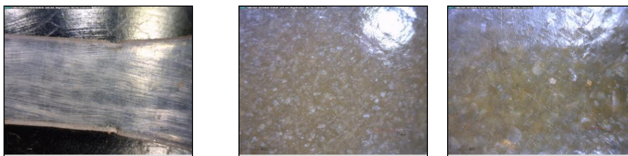
Figure 1. Composites of pure amorphous PLA (left), amorphous PLA + chitin (middle) and amorphous PLA + chitosan (right) at light microscope (50x)
