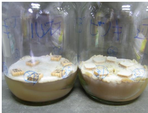
Figure 1. The wood decay test with T. eurrhizus . Strain: T3, samples: heartwood (left) and sapwood (right) of Japanese cypress
