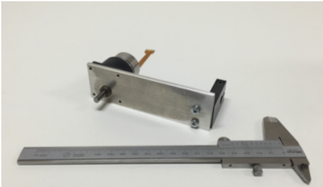
Figure 66: Joint 6 assembly, mounted on link 5 , with motor installed.
