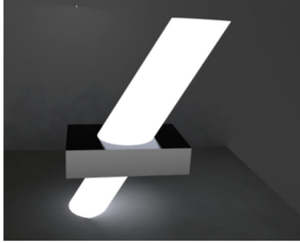
Figure 100: Effect of the mask thickness on the light spot: the incoming sunlight can be partially obstructed by the mask
