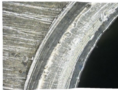
Figure 1.11 Surface texture after the tightening of an hexagonal metric screw over an aluminum sleeve
