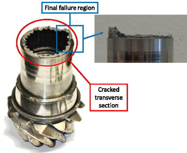
Figure 2.1b Failed pinion shaft
