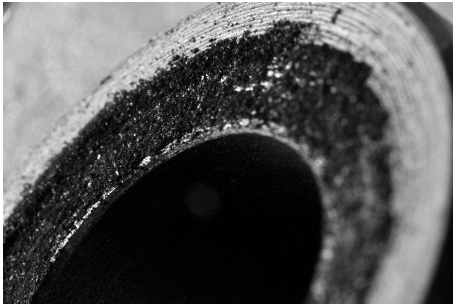
Fig. 3.18 Large amount of iron debris just after five re-tightenings and screw removal
