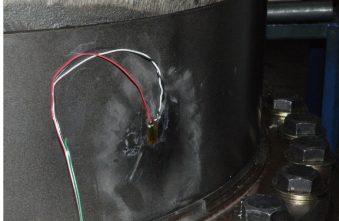
Figure 3.14: Position of the strain gauge at the outer surface of the ring
