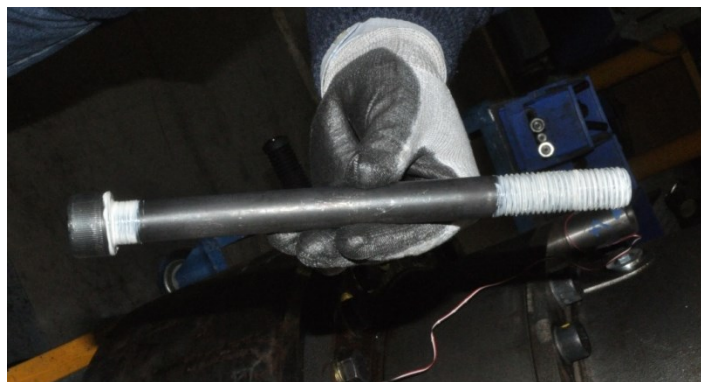
Figure 3.14: Application of the ceramic paste
