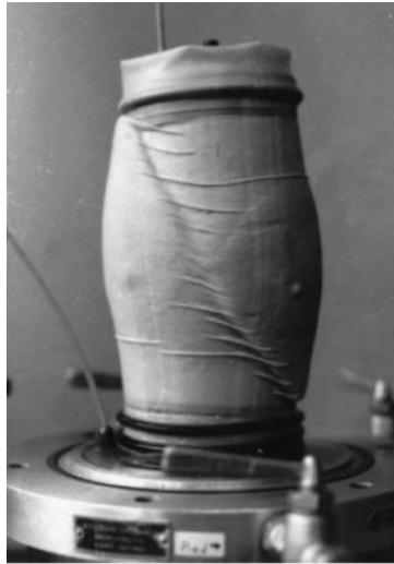
Fig. 2.2 Example of localization with shear plane along a triaxial test; after J.L. Colliat-Dangus Doctoral Thesis, cited by (Desrues & Chambon 2002)
