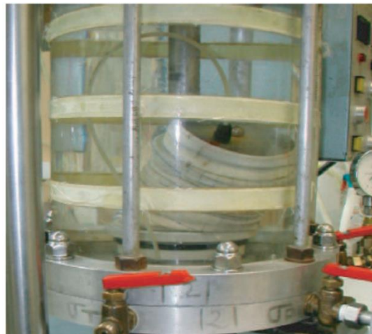
Fig. 2.3 Example of liquefaction after an undrained triaxial test due to a “perturbation” after the deviatoric stress peak q (Servant et al. 2005)
