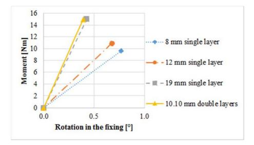
*Fig. 5.* Upper ending rotations in case of different overall thickness HSG (the number means in the marking the thickness of the specimen)
