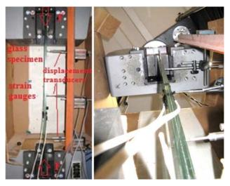
Fig. 2. The first laboratory test set-up and a buckling specimen
