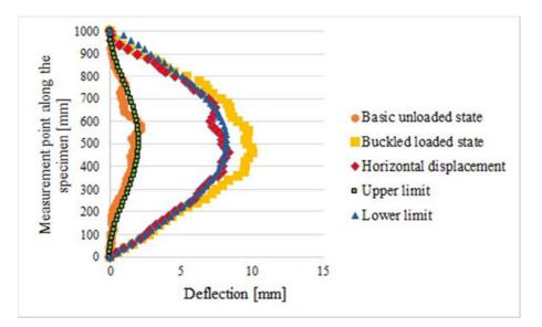
Fig. 7. Deflection measurement results of 8 mm thick glass specimen with partly pinned support
