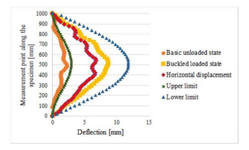
Fig. 6. Deflection measurement results of 8 mm thick glass specimen with partly fixed support
