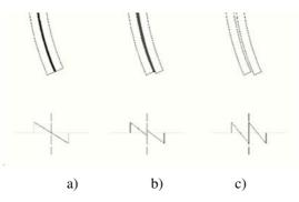
Fig. 8. a) Monolithic behavior, b) real behavior; c) lower (layered) limit
