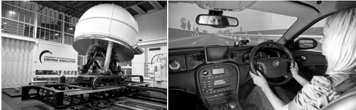
Figure 2. Exterior view (left) and vehicle cab (right) of the University of Leeds Driving Simulator
