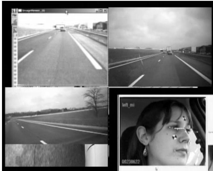
Figure 1. Video sources from: stereo-vision camera with radar for distance estimation to obstacles (top left), the front view (top right), the rear view (lower left – upper part), the view from the left outside mirror down to the surface of the road (lower left – lower part), and the view of the participant's head with the glance direction of the eye (lower right)
