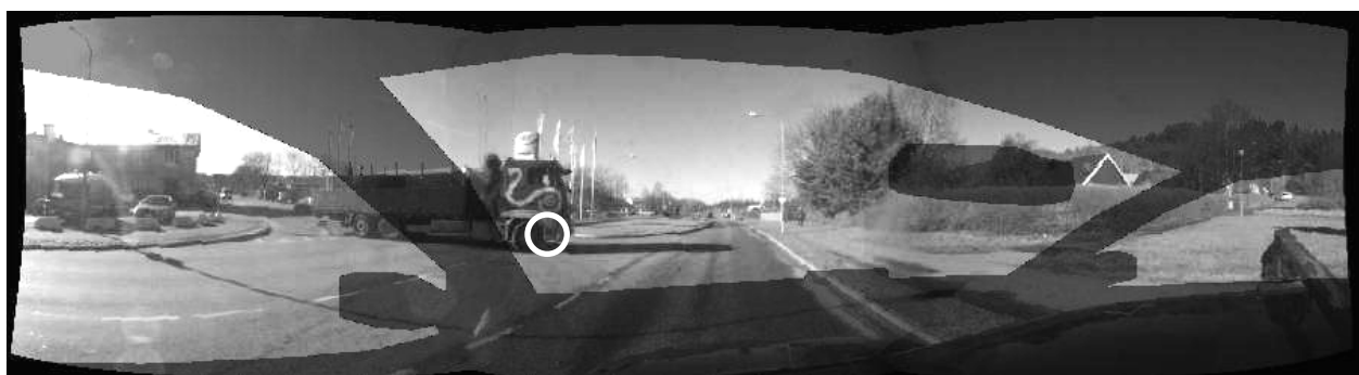
Figure 1. Screenshot from offline visualization tool. Gaze direction from eye tracker visualized as circle
