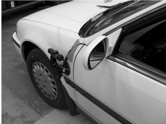
Figure 1. The camera, mounted just below and in front of the left mirror
