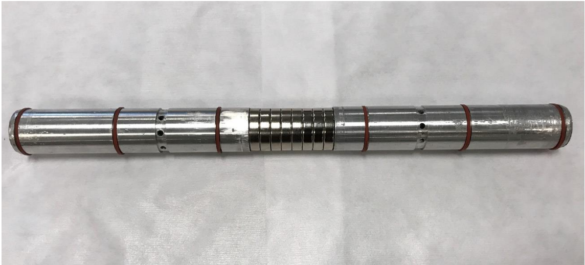
Figure 3.2: The Piston with O-rings (O-rings in red color)
