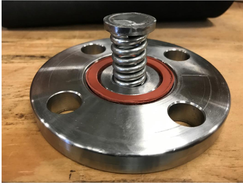
Figure 3.4: The Flange of the Cylinder with O-ring and the Spring-Washer Cap Assembly
