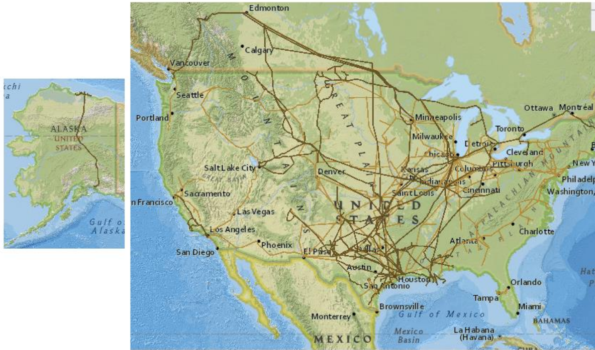
Figure 1-1. Crude oil and petroleum products pipeline systems [3].
