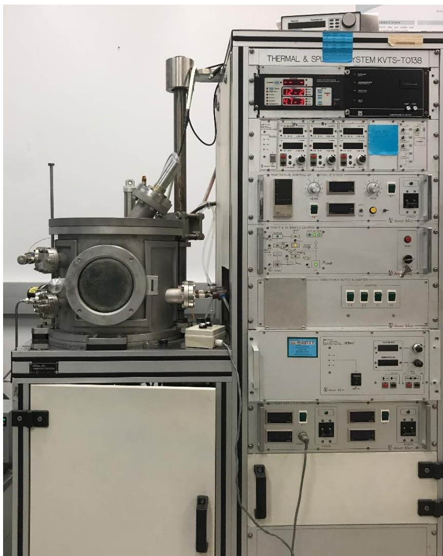
Figure 14: Deposition Chamber (left) and controls (right)
