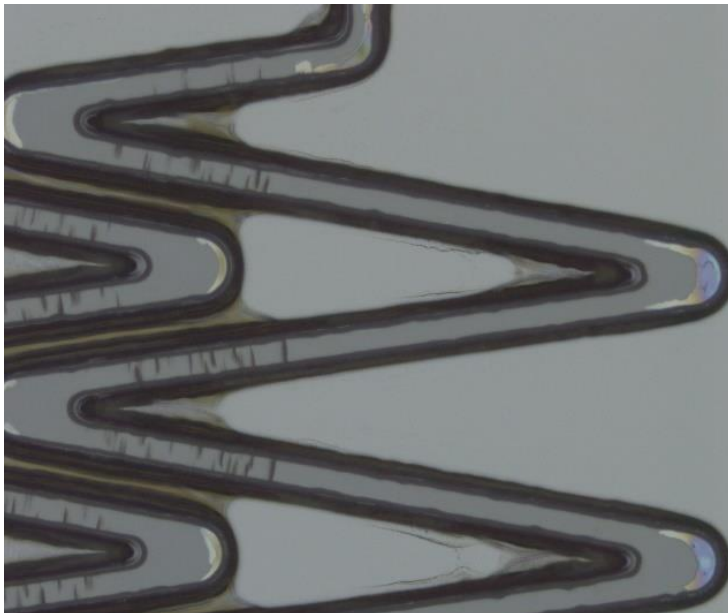
Figure 3: SU-8 features before treatment (The webbing visible due to over exposure does not alter the results of the experiment)
