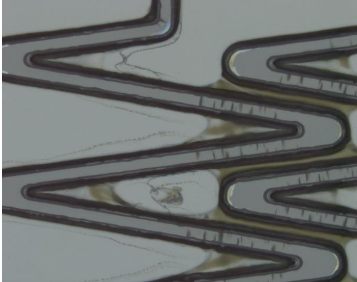
Figure 1: SU-8 features before treatment (The webbing visible due to over exposure does not alter the results of the experiment)
