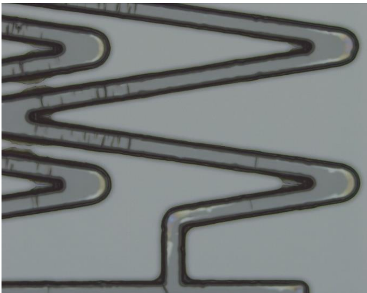
Figure 7: SU-8 features before treatment
