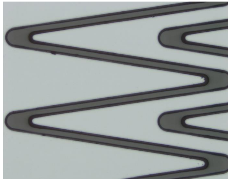
Figure 22: Surface cracks are healed and SU-8 structures
