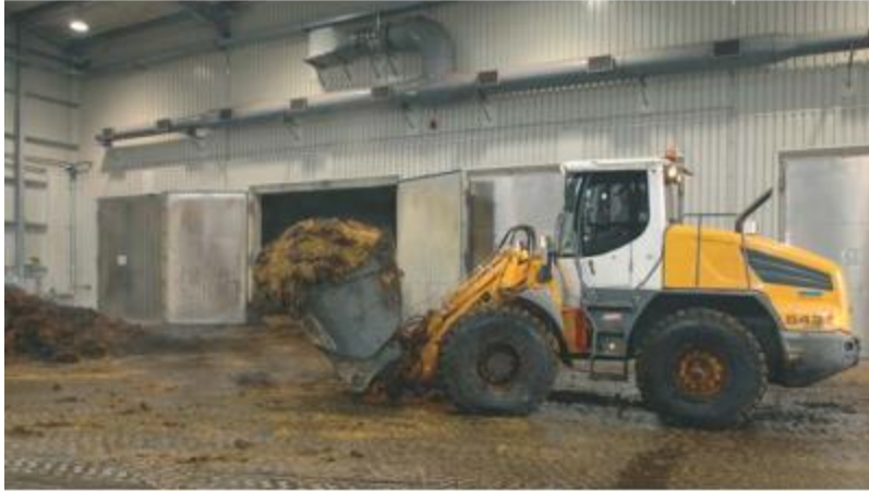
Figure 8. Interior of a BIOFerm Dry Fermentation System.
