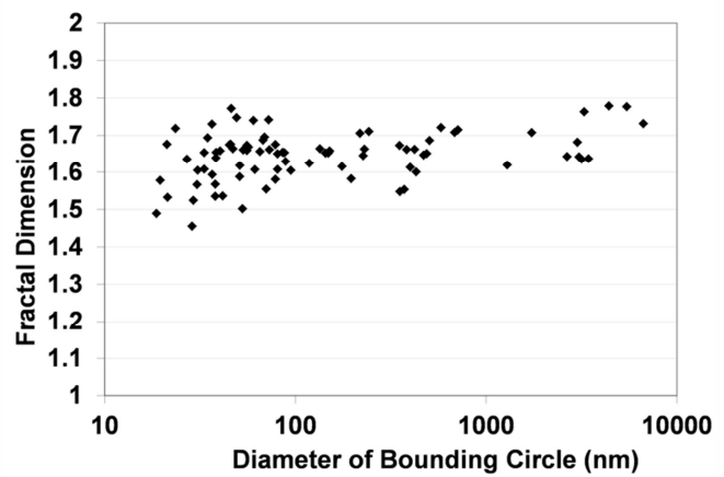
Figure 3-5: Fractal dimension as a function of size for 84 aggregates. Large aggregates possess fractal characteristics consistent with three-dimensional growth.
